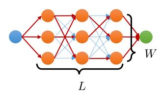
$$f(x) = (W^{(L)}\eta(\cdot) + b^{(L)}) \circ (W^{(L-1)}\eta(\cdot) + b^{(L-1)}) \circ \cdots \circ (W^{(1)}x + b^{(1)})$$
